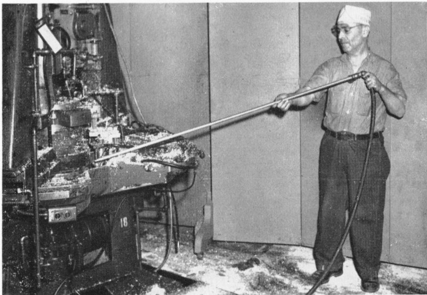
Mike Giudice of the Chucking Department is demonstrating the use of the cleaning device made by that department. This device reduces the hazard of flying dirt and chips when cleaning machines with air.
